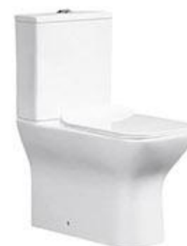
MP-8602 Washdown Two-piece Toilet Flushing system: Rimless Size: 605x370x820mm P-trap: 180mm, S-trap: 100/250mm
